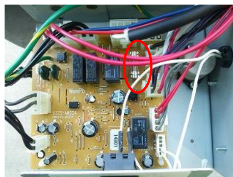
Picture 11 Inspection fuse
