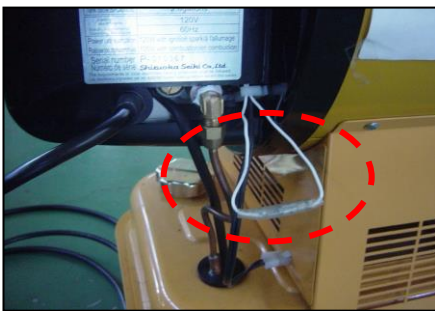
Picture 6 Inspection terminals for control device(PH5)
